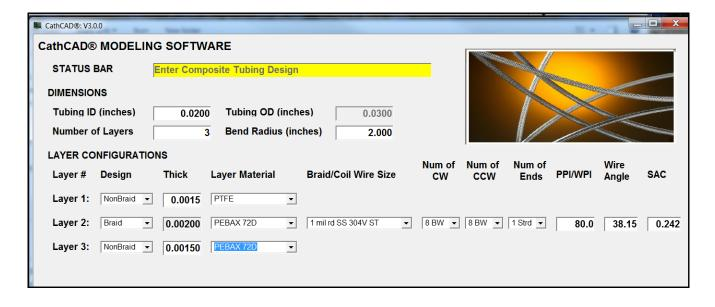
If you know the braid angle of your design but not the Pick Count, you can enter trial values of the pick count into the SOFTWARE until your desired braid angle shows up on the screen. The computation from Braid Angle to Pick Count is nearly instantaneous.
