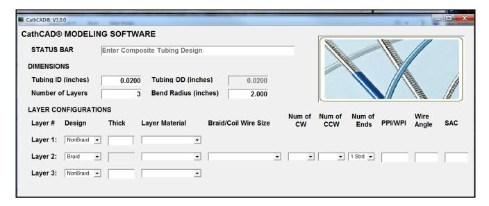
The screen shot below shows the three layer composite tubing design after being completed by the User.
