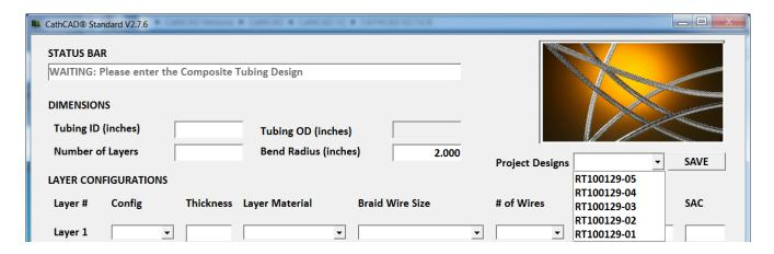
In order to RELOAD a project design, select the applicable project design from the drop down dialog box located next to the Project Designs title on the data entry form. The SOFTWARE will ask for permission to reload the design before proceeding.
