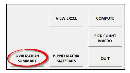
The function graphically summarizes the major and minor diameters of the design as a function of bend radius as shown. The results may be exported directly to Microsoft Excel (which includes the numerical results) for further review.
