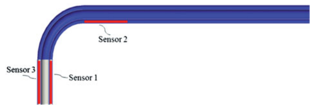
Figure 5. Possible configuration of sensors. Sensor 1 and 2 are positioned according to the method proposed in [11]. Moreover, Sensor 3 is integrated into the catheter tip as a precautionary measure to refine catheter calibration.
